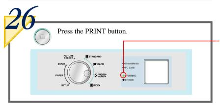
The lamp flashes when the PRINT button is pressed after which printing begins.
